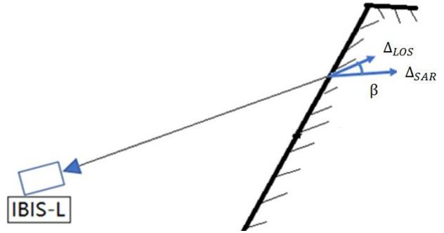
Fig. 15 LOS-displacement and real displacement (Hassan et. al., 2018)
