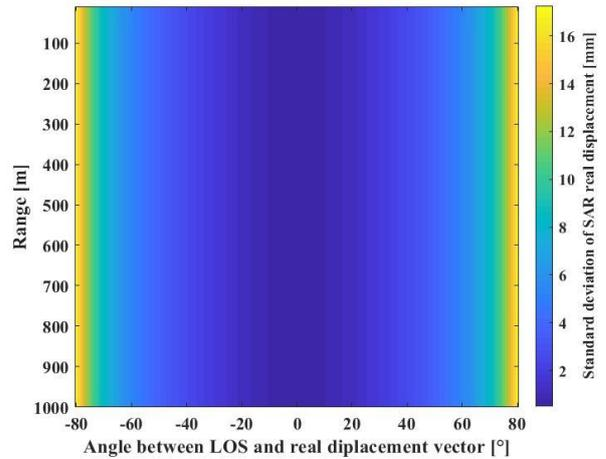
Fig. 18 Standard deviation of the real SAR-displacement for the first scenario
