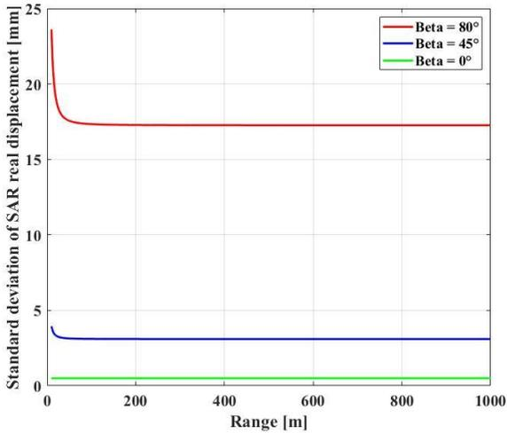
Fig. 20 Standard deviation of the real SAR-displacement for the second scenario along the whole range and under different  $\beta$  angles
