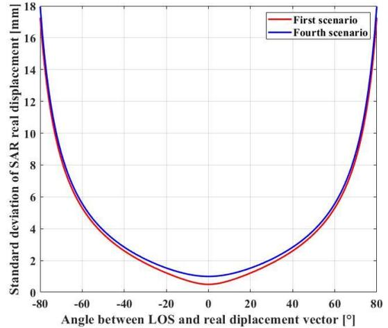
Fig. 22 Standard deviation of the real SAR-displacement for the first and the fourth scenario at 500 m range
