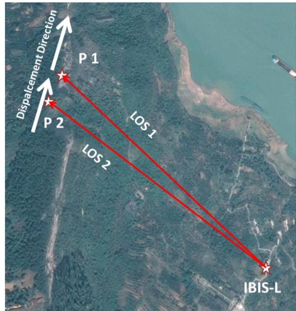
Fig. 24 Measurement configuration and the direction of the expected displacement
