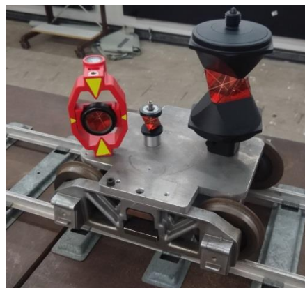
Fig. 4 – Miniature trolley with the used reflectors (from left to right: Leica Miniprisma GMP111, Leica 360° Miniprisma GRZ101, Leica 360° Prisma GRZ122)
