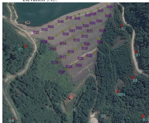
Fig. 3 Pilasters and monitoring markers
