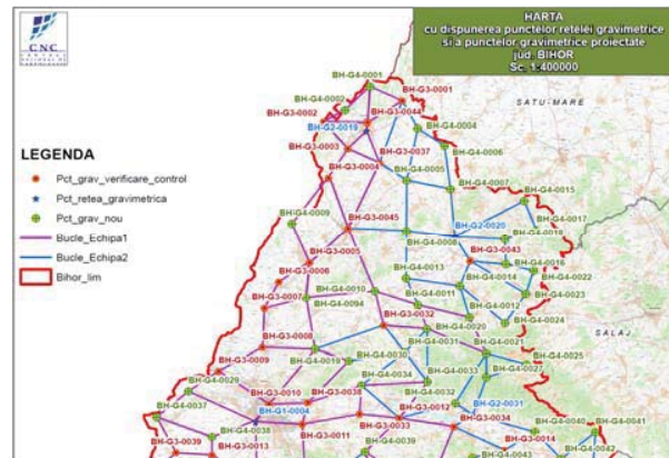
Fig. 1 The layout of the gravimetric points in the pilot project from Bihor County
