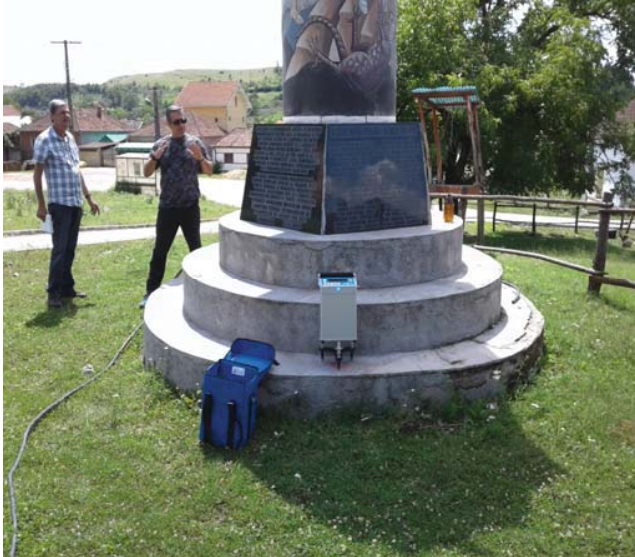
Fig. 2 Performing gravimetric measurements in a new point of a loop
