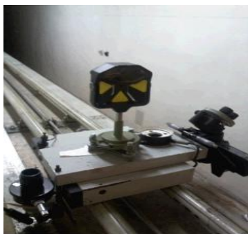
Fig. 3 Measuring trolley and support.
