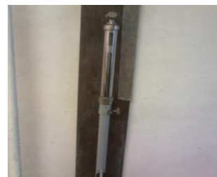
Fig. 2 Barometer is located in the geodesic base to monitor atmospheric pressure.
