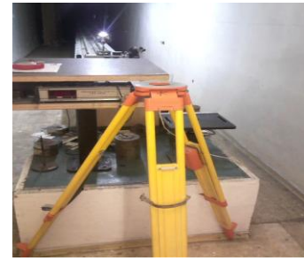
Fig. 5 The way of measuring mobile trolley at the point, " 0 " m the geodetic base
