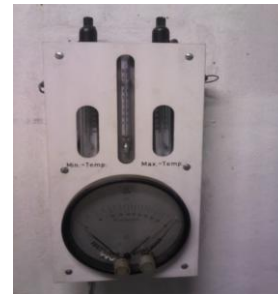
Fig. 1 Thermohygrometer. It is located in the geodesic base to monitor temperature and humidity.
