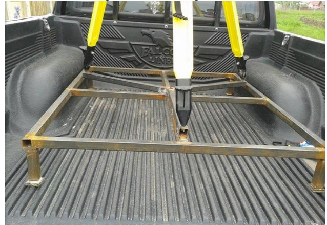
Fig. 6 The position of the tripod on the metal frame
