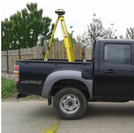
Fig. 5 The vehicle equipped with the measuring instrument
