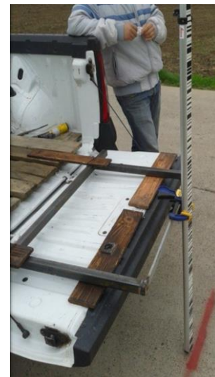
Fig. 7 The gripping system for placing the rod at the back of the vehicle
